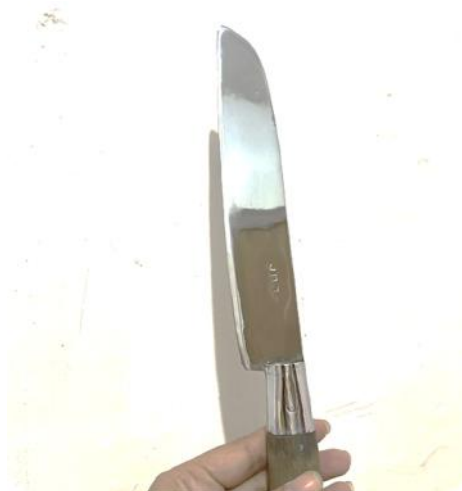
Gambar 3. Pisau hasil proses Electroplating Chrome
