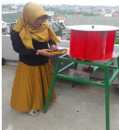
Gambar 5. Uji Coba Vertical Axis Wind Turbine Type Savonius
