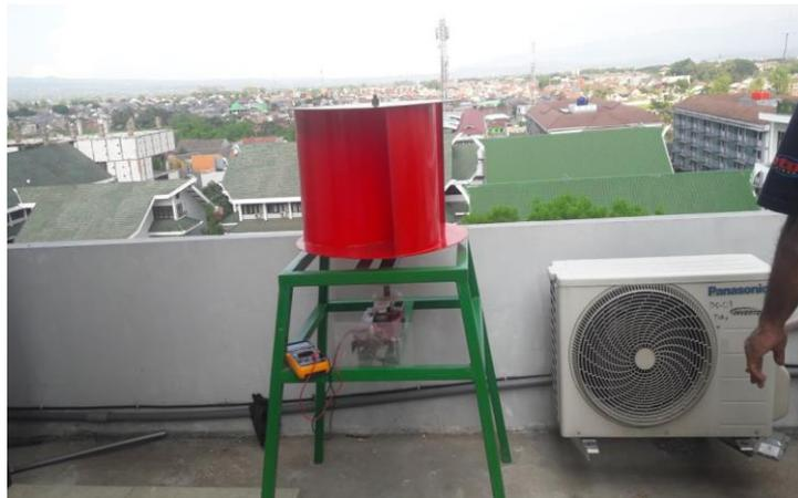
Gambar 4. Vertical Axis Wind Turbine Type Savonius
